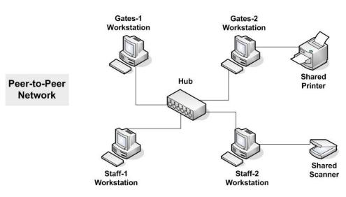
Shown above, there is a scanner that is connected to the Staff-2 Workstation, this scanner can be shared with the other workstations connected to the networking. Similarly, the Gates-2 Workstation has shared its printer.
